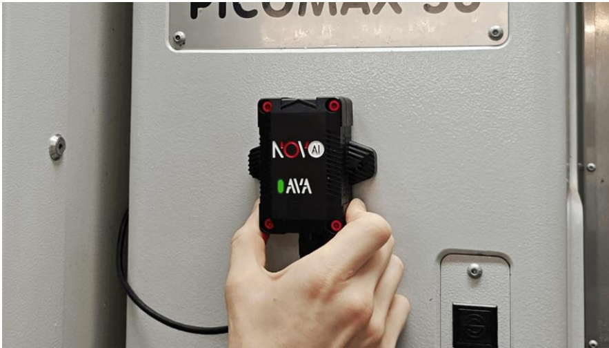
Retrofit in practice: an external AVA sensor on an existing machine.
